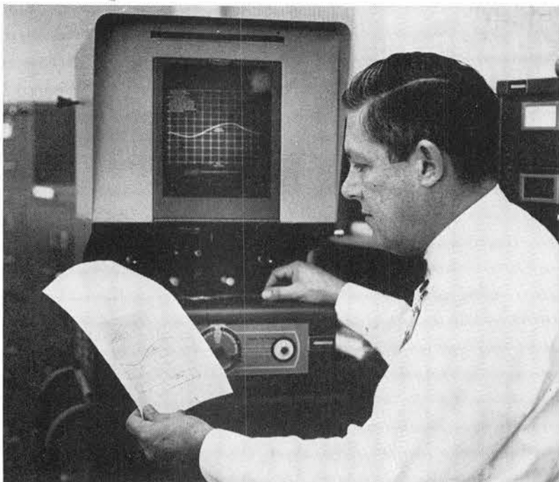
FRESH PRINT from microfilm containing environmental testing data is checked by Dick Corn (7185-3). IBM cards with the microfilms and additional information are filed in the drawers to the right for the later use of designers and others when needed.
