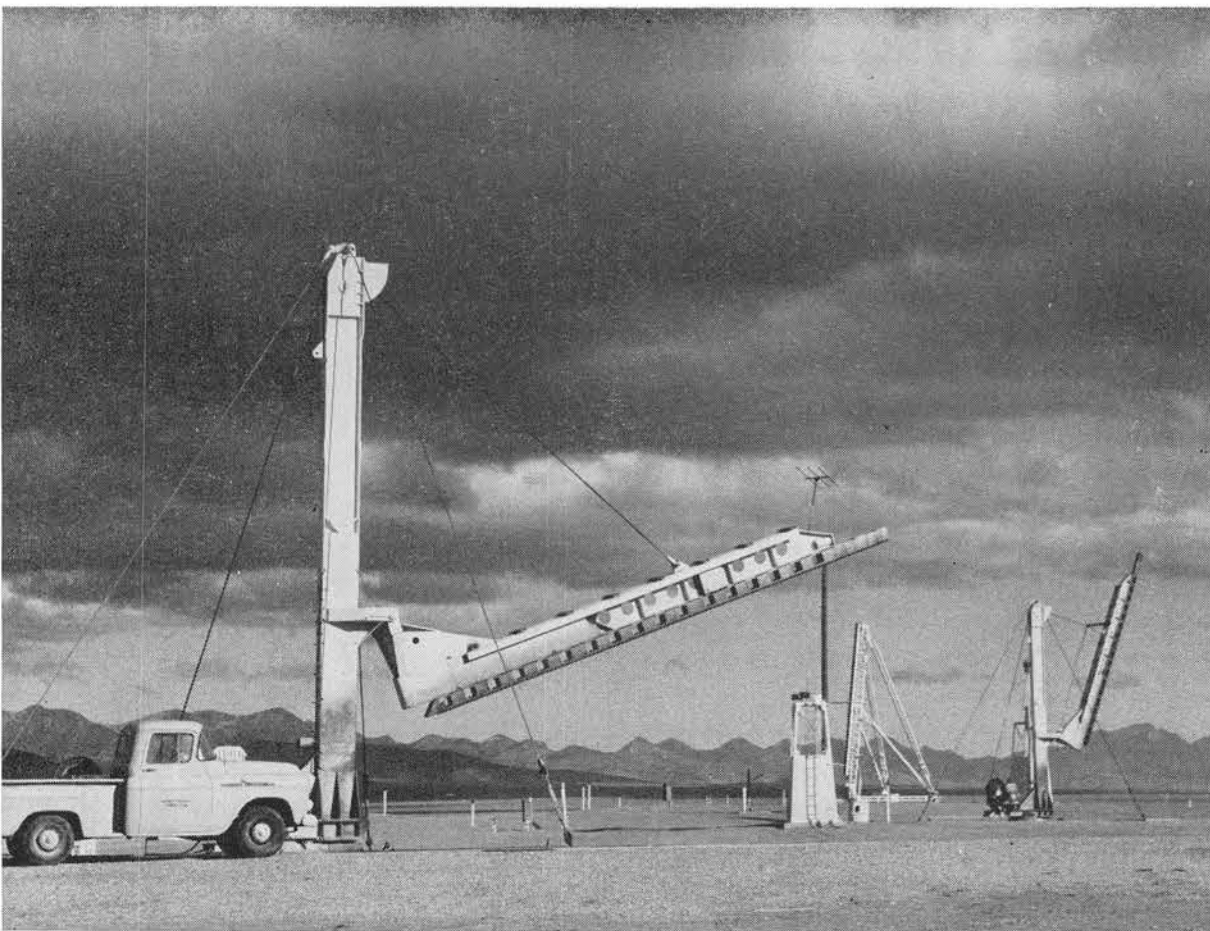
THREE ROCKET LAUNCHERS are part of the launch complex at Tonopah Test Range. In the foreground are two NASA type launchers used by the Mach 5 and Supersonic Parachute Test Vehicles.
