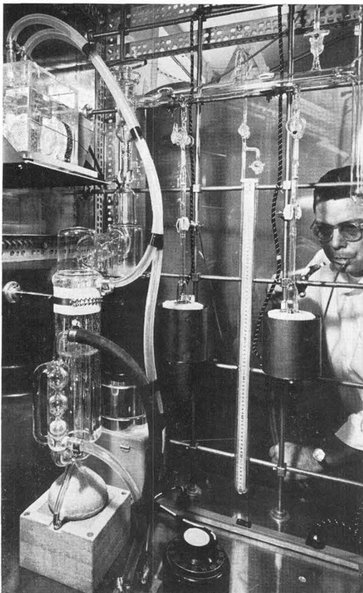
FINAL ASSEMBLY of an intricate glass vacuum system fabricated by Sandia's Glass Shop 4224-5 is made by Warren Roberts in the laboratory area of Division 1411 in Bldg. 817.
