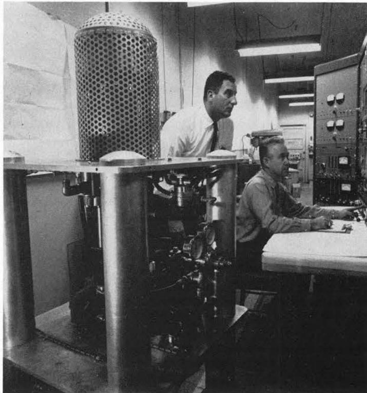
SANDIA PULSED REACTOR (minus fuel material) is shown at left while operators P. D. O'Brien and J. C. Conant (both 5431-2) are observing control console. The reactor will be located in a concrete hemispherical reactor building in Area III. This picture was taken in Bldg. 839 where the equipment was assembled.
