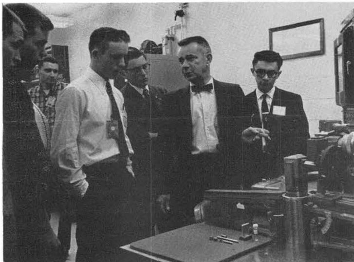
AN X-RAY DIFFRACTOMETER, used to analyze elements in materials, is explained to several chemistry students by B. K. Seely (1122) during the Edison Day Tour last Friday at Sandia Lab.
