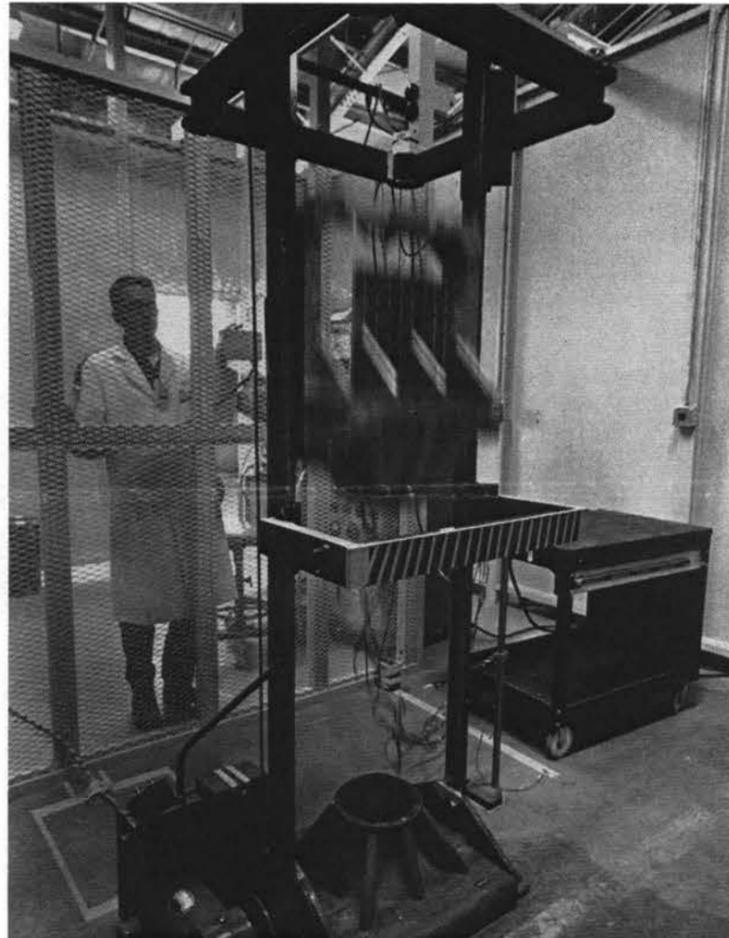
BLURRED CARRIAGE in this drop will impact on rubber to produce a half-sine shock pulse input to the component secured to the carriage. Operator is K. R. Ludwick. This Barry drop tester features a catch mechanism which will prevent successive bounces.
