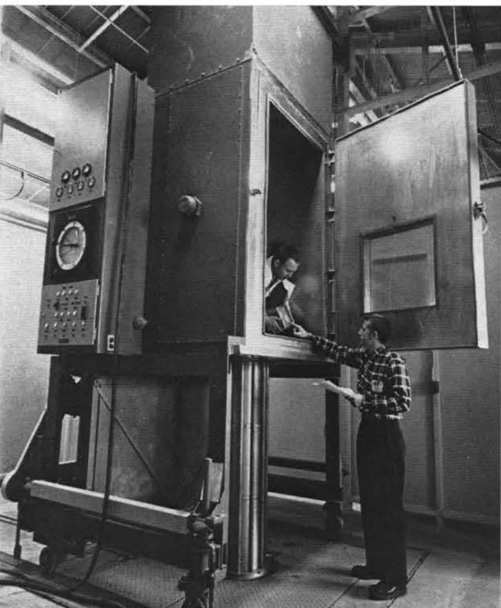
COMBINATION temperature-mechanical shock apparatus is readied for use by B. B. Conklin (in chamber) and R. O. Brooks. Test units can be heated to 500° F. or frozen to minus 100° F. and then shocked from the actuator tube running from the chamber to the floor. Machine can produce from 300 to 500 g's shock.
