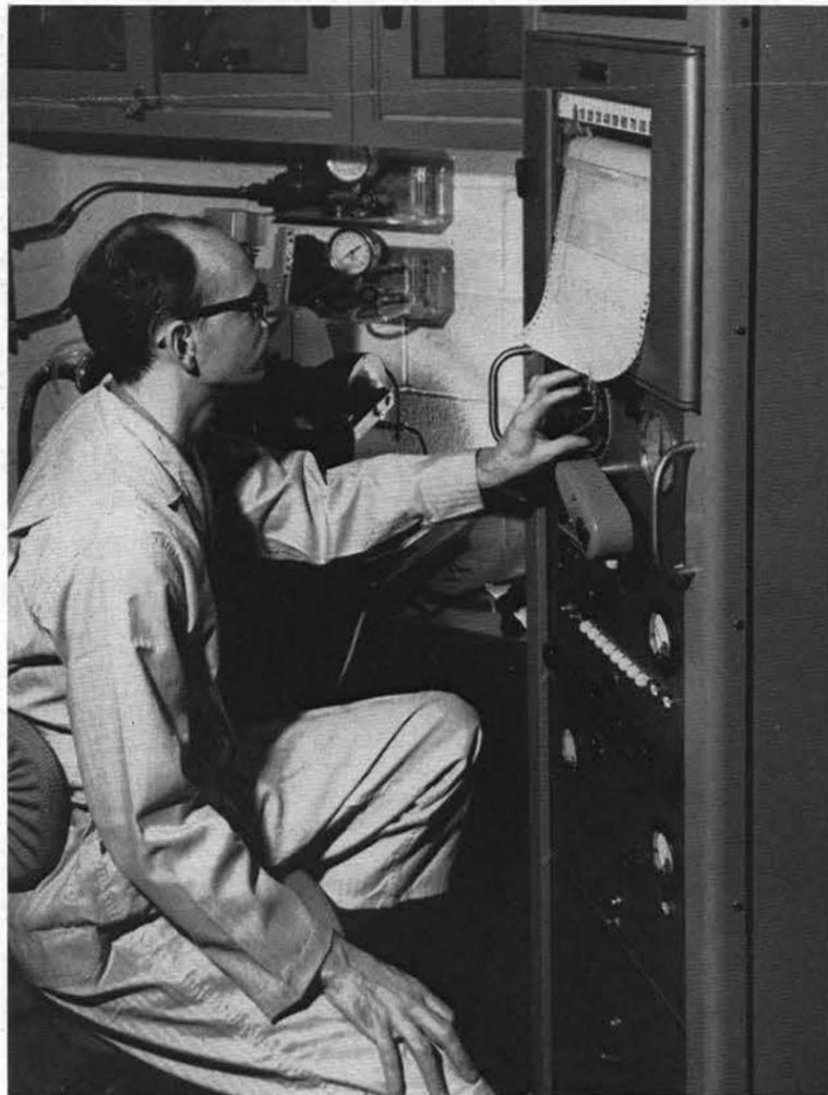
**X-RAY SPECTROPHOTOMETER**, operated here by Lee Klaus, can identify most any substance from only a few milligrams.
