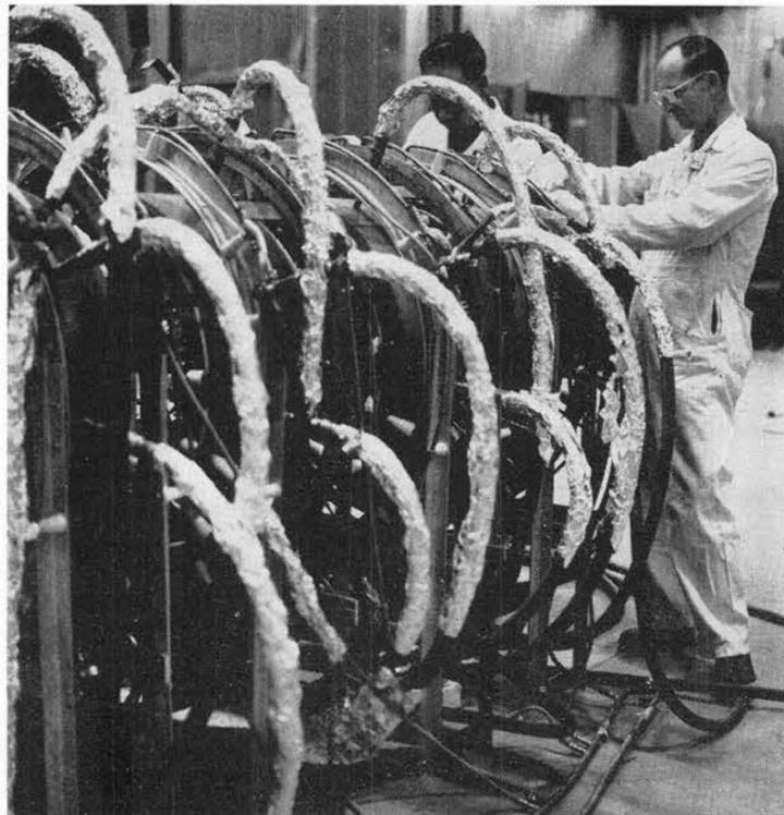
**INTENSE HEAT** makes necessary insulation and cooling measures in the radiant heat facility. Working on the unit are J. E. Breitenbach and James Brandolino of High Temperature Section 7323-4.
