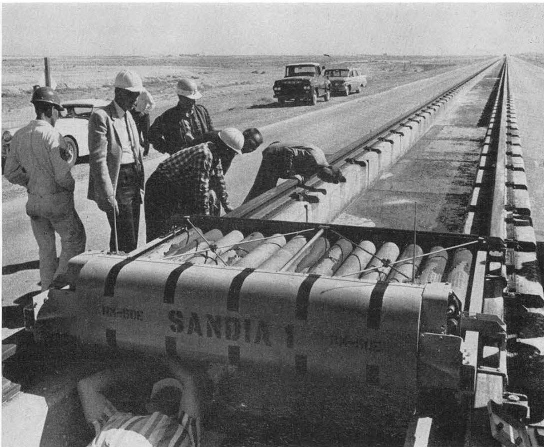
SEVERAL SANDIANS inspect a sled following its run on the six-mile Holloman sled track. The rocket sled reached a velocity of 1300 feet per second (885 mph) before coasting 11,838 feet to a stop.
