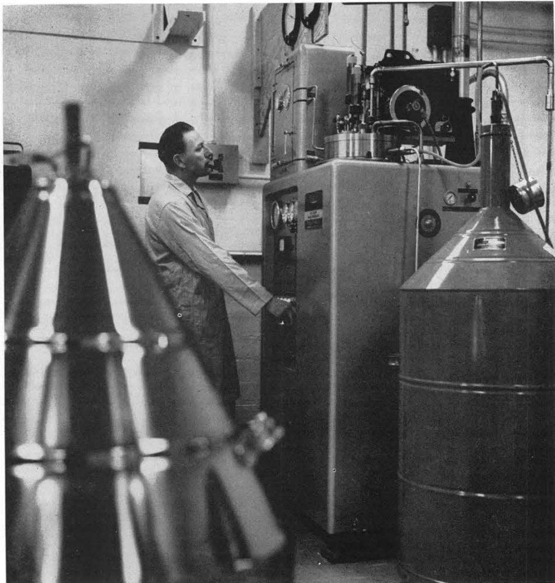
THIS ADL-COLLINS helium refrigerator, installed in Bldg. 855 last month, is used to achieve a near-perfect vacuum for materials testing. Ray Drury (1413-2), who will operate the machine, is checking temperature gauges. In the foreground are two Dewars containing liquid air for pre-cooling helium.
