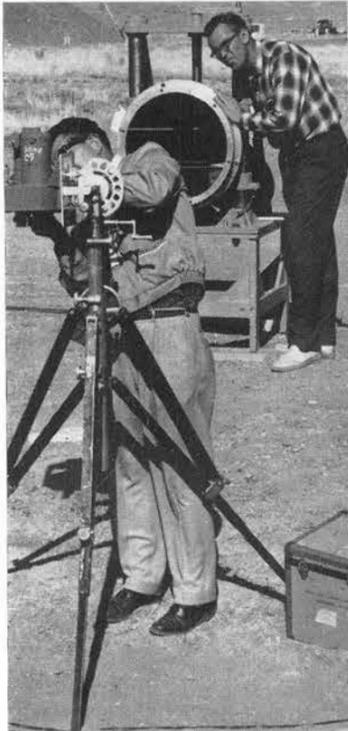
A HIGH-SPEED CAMERA, using a shadow graph technique, will record shock waves created when a test vehicle is shot down the rocket sled in Area III. J. H. Banker, foreground, and D. L. Fastle (both 7244-2) are shown adjusting one of the two mirrors which are used to get a collimated beam of light across the track.
