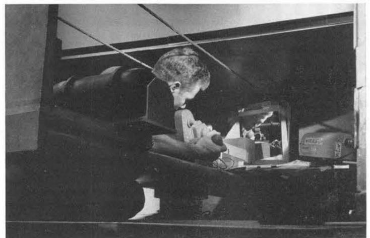
DICK GRAY (8123-3) adjusts Fairchild camera on centrifuge boom before shooting environmental test at Livermore Laboratory. The mirror (rear) is used in filming the opposite side of the test device. The Fairchild camera operates at 64 to 8000 frames a second and the Milliken camera (right) shoots at 400 frames a second.
