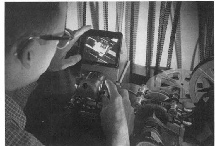
PAUL VAN DYKE (8123-3) uses film editor to view close-up of microfilm feed mechanism on a reproduction machine. Films Paul shot of the machine in operation revealed a malfunction in the machine and led to its correction by the manufacturing firm.
