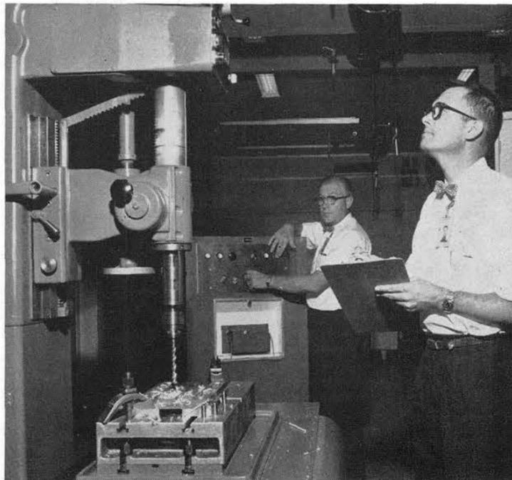
EVALUATING a numerically controlled drilling machine are E. S. Roth (foreground) and A. R. Konecny of Advanced Manufacturing Development Section 2564-1. The machine is automatically controlled by the computer-like console operated here by Konecny.
