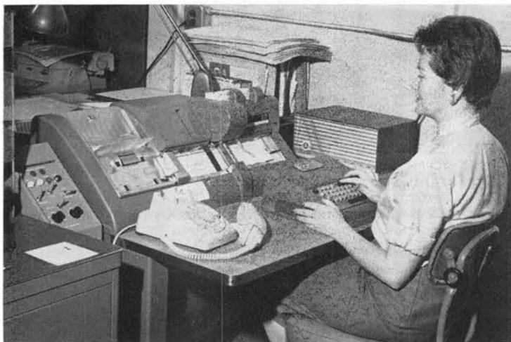
**IN BLDG. 887**, Mary James (4613-1), by pressing a button, can make duplicates of order cards Dave Sample has just sent in. Data on the IBM prepunched cards are transmitted over regular telephone lines from stockrooms at Sandia Laboratory to Bldg. 887.
