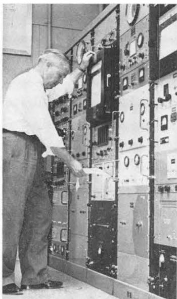
**FREQUENCY STANDARDS BANK** in Bldg. 861 is operated by Howard Burgess (2412-1). Five oscillators produce 100 kilocycle signals which are inter-compared plus a daily comparison made with the standard frequency broadcast by the National Bureau of Standards. Accuracy is five parts in  $10^{10}$ .
