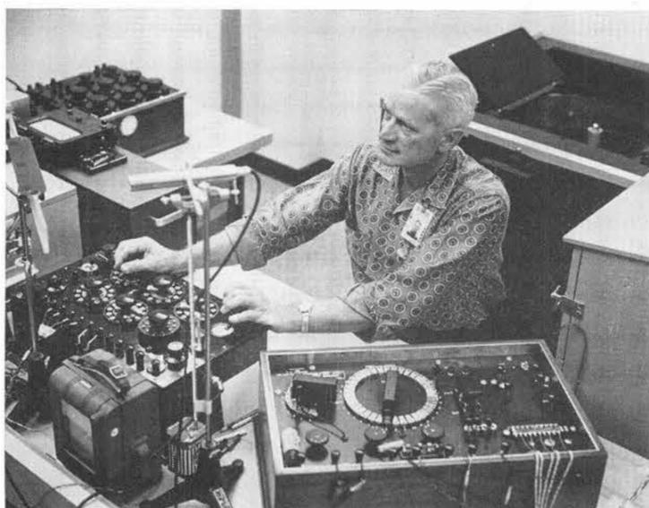
**MONITORING** temperature of oil bath in background which contains the Primary Lab's standard cells, Neile L. Hensinger (2412-3) prepares to certify standard cells used by secondary labs. The temperature is maintained at  $28^{\circ}$  within plus or minus .001 of a degree. In the foreground is a standard potentiometer which is used in intercomparing standard cells with primary references.
