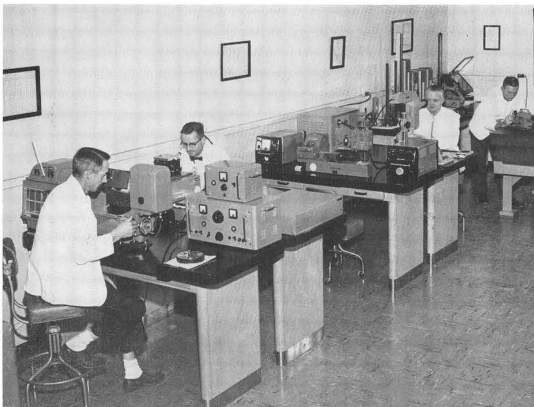
**LENGTH AND MASS** measurements laboratory is housed in a humidity and temperature controlled room in Bldg. 860. The section personnel perform standards measurements of mass, length, angles, circular, profile, roundness, straightness, flatness, squareness, surface finish, screw threads, and gears. From left, above, are Oran May, Joe Moody, Frank Anderson, Errol Gay (all of 2411-1).
