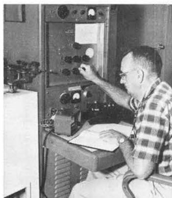
**INSIDE** white chamber above is a glass leak standard. The instrument, a standard leak calibrator, operated here by A. B. Lawrence (2411-2), determines the amount of helium gas escaping from the glass cylinder. Accuracy is within two microns.
