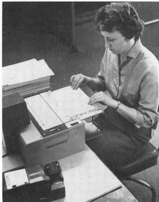
**PERSONNEL RECORDS**, vital documents, and Technical Library manuals are photographed on 16mm film by this Recordak camera operated by Bonnie Smith. Special feature is the complete film unit which attaches to the camera. An average of 2300 shots is taken on 16mm reels each day.
