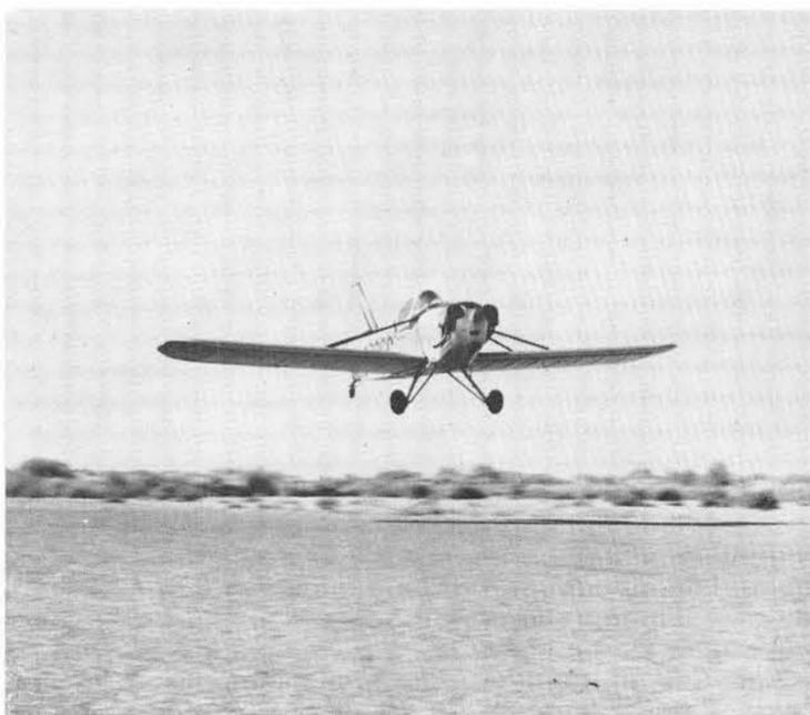
WHIZZING OVER the Seven-Bar runways, Lew Longmire logs more test time in his homebuilt airplane. Made of hardwood, plywood, fabric, and a little aluminum, the plane weighs only 750 lbs. with Lew and a full tank of gasoline aboard.
