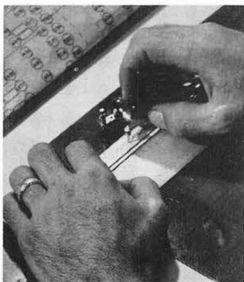
**OLD METHOD** of numbering electrical circuit boards at Livermore Laboratory was done manually using this special lettering pen. Information was copied directly from engineering drawings and took up to two and a half days to complete.
