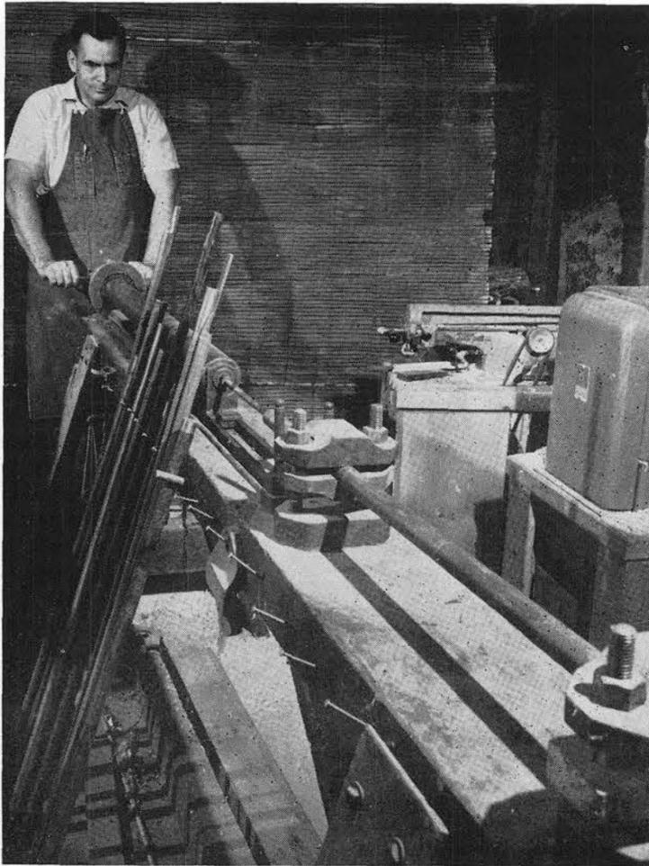
PATIENCE is a virtue in hand-boring muzzle-loading rifles. Dick Hicks uses boring machine he built to Colonial period specifications.
