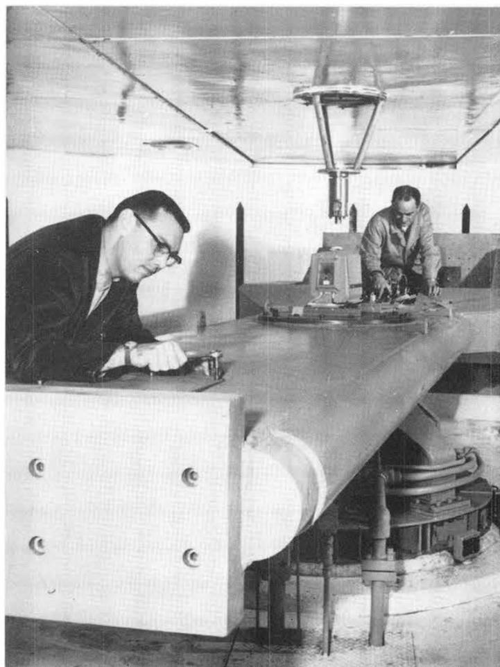
FINAL ADJUSTMENTS on Livermore Lab's newly-installed centrifuge are made by Harry Jacobs (8121-2), foreground, and Bill Maxwell (8121-1). Mounted in the center of the boom is a closed circuit television camera which will enable engineers to view test components while the centrifuge is in motion.
