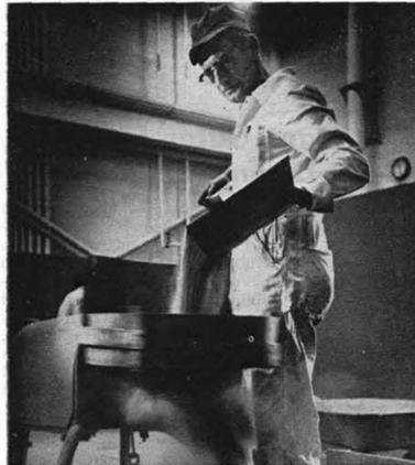
"RIDDLING" SAND, Donald Quayle shovels the special Foundry sand through a vibrating screen called a sand riddle prior to forming a new mold. Sand is continually re-used.
