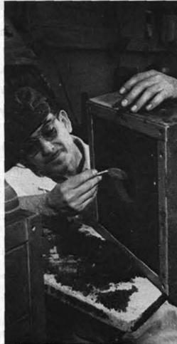
SMALLER PIECES for foundry casting are prepared in small "bench molds." Here Ramon Armijo smooths section of mold.
