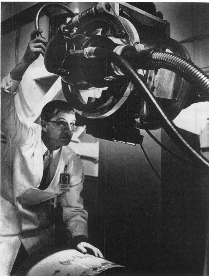
ADJUSTING 25-kilovolt X-ray generator, S. A. Ravenbyrne prepares to make an exposure of a large metal casting prepared by personnel of Sandia's Pattern and Foundry Section 4221-4.
