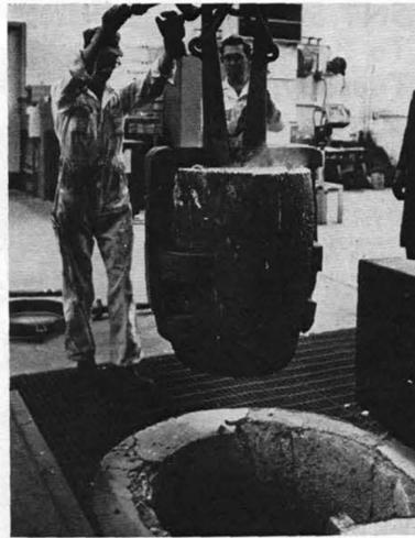
CRUCIBLE of molten aluminum is lifted out of the furnace by using overhead crane. Performing the operation are Donald Quayle, left, and Wilfred Sanchez. Sandia furnaces do not have large exhaust hoods over the furnaces that are common to most foundries, instead a steady stream of air is blown across from duct at left, sucked out by a duct on right.
