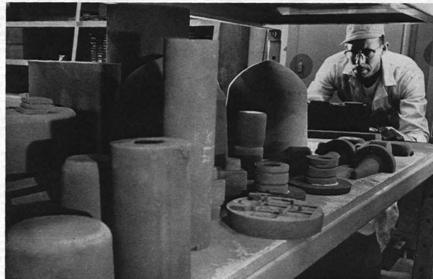
UNLOADING CORE OVEN RACK, Manuel Martinez checks a typical day's production of sand cores. Cores will be placed in molds for next day's schedule of pouring. Cores are produced from wooden patterns.
