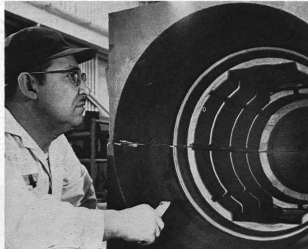
OUTSIDE CORE for a wind tunnel section is prepared by Candelario Torres. Core was made in two sections, baked and assembled. Finished piece weighed more than 1000 lbs. It will withstand tremendous temperatures and strain.
