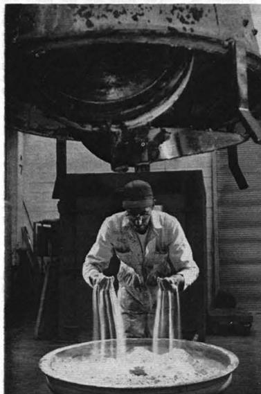
LINSEED OIL and Bentonite are added to the Foundry sand for use in forming cores. Here Manuel Martinez checks "feel" of the mixture. Nearby machinery is a sand muller which fits on top of the round sand basin. The blades revolve to thoroughly mix the sand. In background is pictured the electric core-oven.
