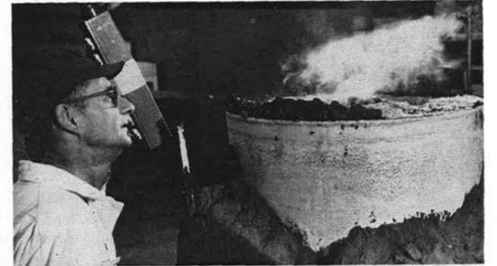
STILL-HOT CASTING emerges as the sand of the mold drops away. Small rod-like element sticking out of sand at left is one of the "down sprues" through which the molten metal flowed through to the "gate" in the bottom of the mold.
