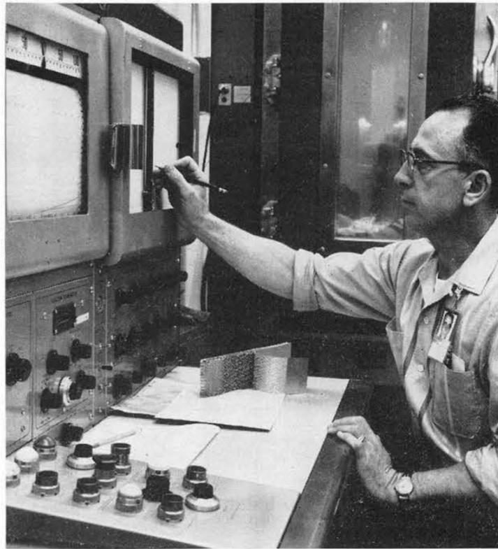
LOW-TEMPERATURE test of foam sample is conducted in chamber by R. L. Buckner (1113-1) in Mechanical Properties Lab.
