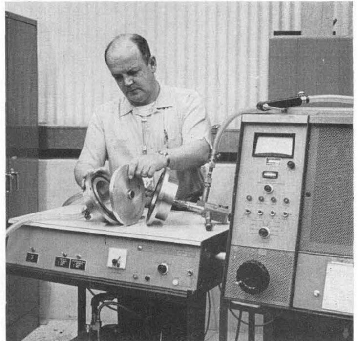
J. R. "BOB" MARTIN (8121-2) prepares metal "hats" for leak detection tests. Item to be tested can be seen in center of metal separator disk which will be enclosed by the hats shown at the sides of the disk. Hats are then bolted together; one filled with tracer gas and the other evacuated. Any gas passing through the test material will be drawn into leak detector (right).
