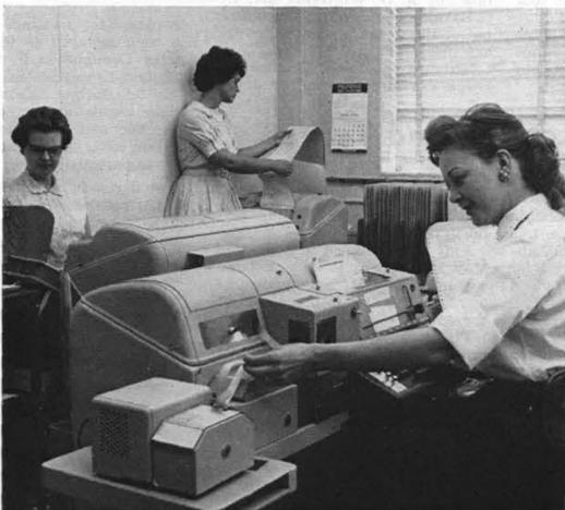
**28ASR TELETYPERS** are used to transmit purchase requisition data to purchasing organizations through the medium of paper tape. Wanda Cupp and Glenna Mosely, foreground and left, operate Teletype transmitters while Juanita Van Jelgerhuis, center, examines a reply at Teletype receiver.
