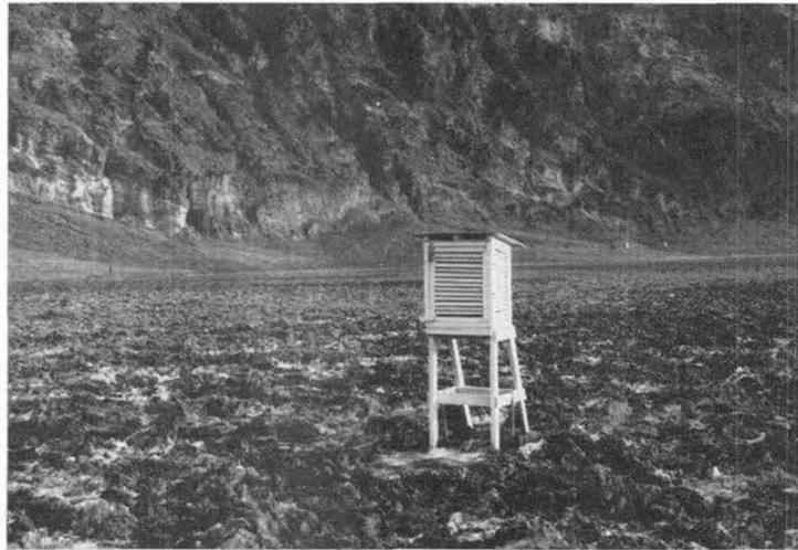
**ISOLATED RECORDING STATION** in Badwater, California, has obtained important temperature data indicating that it is located on the hottest spot in North America. The data is being used in studies aiming at establishing the highest temperatures nuclear weapons have to withstand in desert storage environments.
