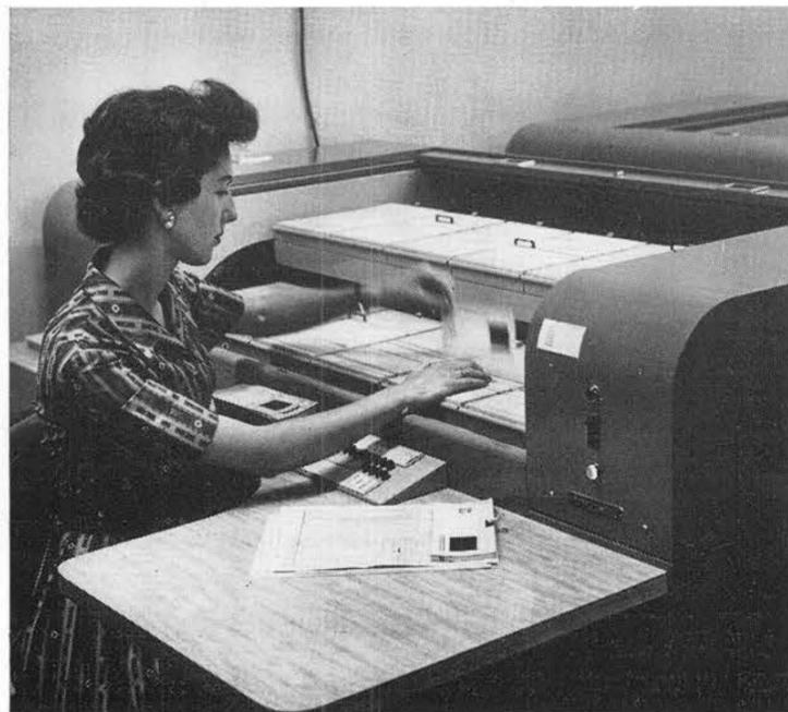
COMPLETED microfilm drawing card is inserted in a rotating-drum file by Carolyn Kinsey of Reproducible Files Section 3446-2. Similar storage facilities are used at film banks located at four Sandia Laboratory locations and at other contractors' locations.
