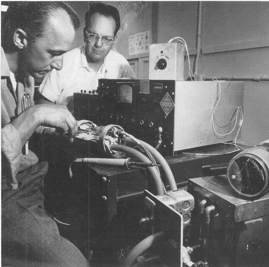
EXPERIMENTAL EQUIPMENT used in calibration study at various reactors throughout the country is checked over by R. W. Healy (left). Asher Kantz used foils of sulphur and plutonium to determine average neutron energy, and silicon for a second study. Both men work in Division 5311.
