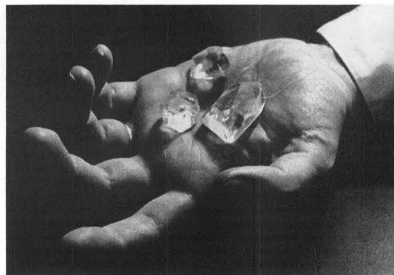
SINGLE CRYSTALS of triglycine sulfate, which have been grown in Section 1124-3's laboratory, are shown in this photograph.
