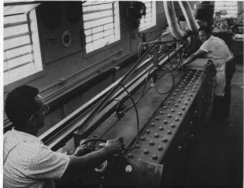
"STONE SAW" in Metal Stock and Cutting area can accommodate pieces of metal up to 12 ft. in length and four inches thick. Phil Moya (right) is measuring aluminum stock two inches thick, while Pedro S. Ortega (both 4212-2) stands ready to operate controls for making a straight cut. Forklift is used to move metal.
