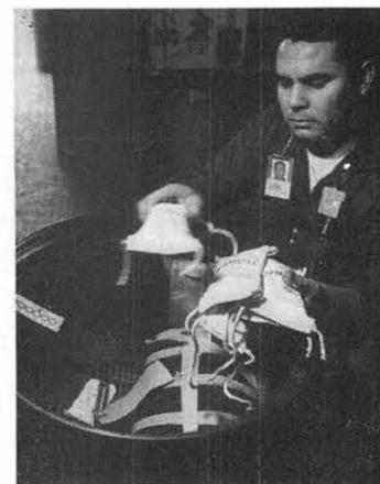
SACKS of desiccant are packed around electronic gear destined for long-range shipment by Gabriel Chavez (4624-2). They'll absorb stray moisture in metal packing container, reduce chance of possible humidity contamination.
