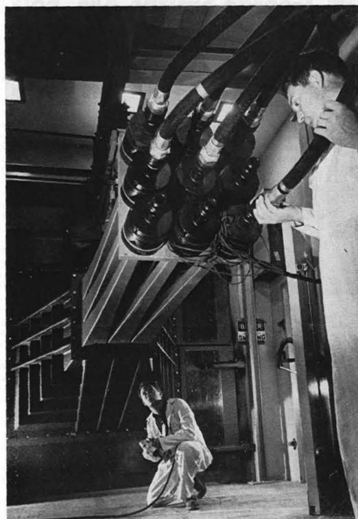
SOUND can cripple components or systems not designed to withstand acoustic stresses. The giant horn above, located in 7300's Area III Acoustic Facility, can produce vibrations that will seriously damage material. John Windsor, center, checks maintenance and John Colburn, right, attaches hoses to supply compressed air to driver during operation. Both are members of Sandia Laboratory's Vibration Division 7324.
