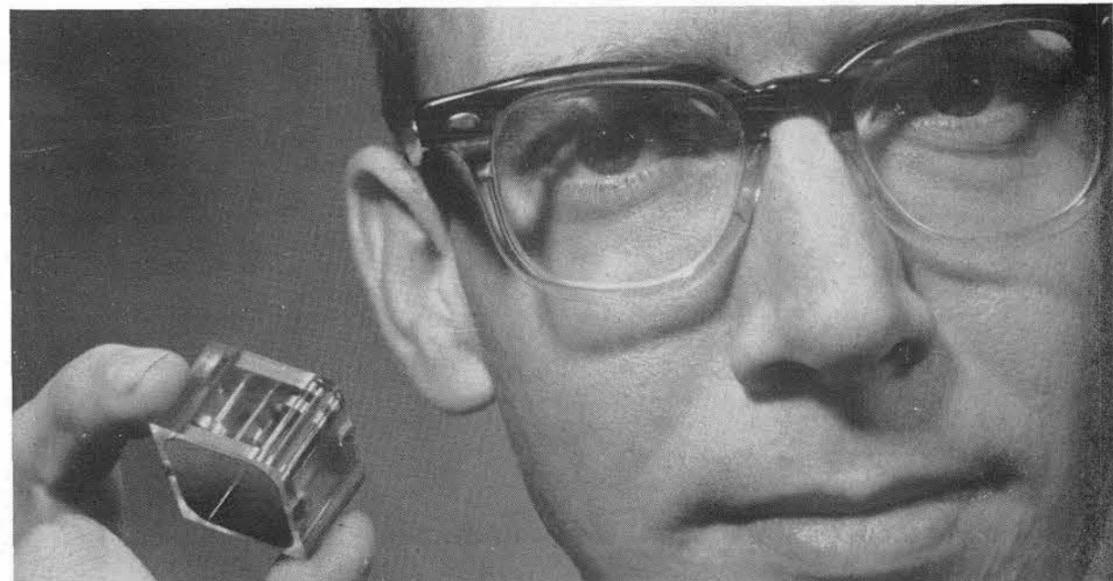
SPECIAL PROJECT, conducted by TDP student Dean E. Gladow (7224), produced 1000-to-one power-reduction unit used five Mylar belt stages instead of gears. in a volume less than one cubic inch. Tiny prototype
