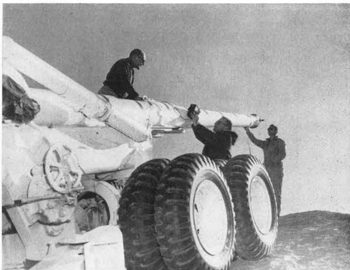
CHECKING STRAIN GAGE instrumentation on barrel of 155 mm gun are Ed Healey, Art Thomas, and Jim Shindelar, all of 8121-4. The gages, placed two-feet apart along the length of the barrel, will obtain data on the acceleration of projectiles fired through the cannon barrel.
