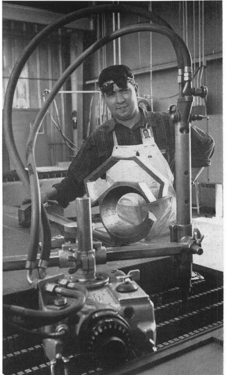
OXYACETYLENE CUTTING TORCH was used by Richard C. Gonzales (4212-2) in displaying a truncated cone shape, various degrees of bevels, different radii and other cuts possible from four inch thick "boiler plate." Tolerances are .0625 to .2500 in. depending on cut.
