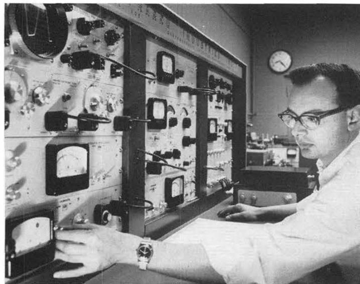
INFRARED DETECTOR CONSOLE is used by Gene Aschettini to analyze performance of various optical detector devices reacting to visible light, ultra violet rays and infrared. A built-in "blackbody" in the console gives a precisely known standard to measure device performance.
