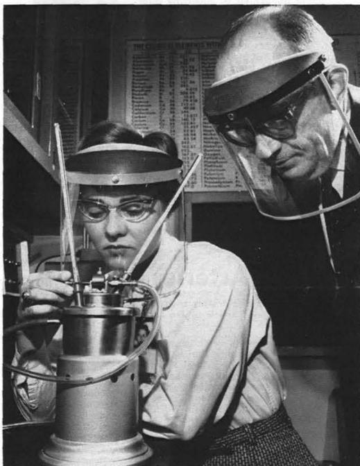
FLASH POINT of highly volatile liquids is determined by Mina Carnicco (3211) through use of a tag closed cup tester as Safety Engineer J. E. Baylor (3210) looks on. Thermometers indicate heat rise of sample and water bath in cylinder. Proprietary products containing acetone or various alcohols are among liquids tested in container such as this.
