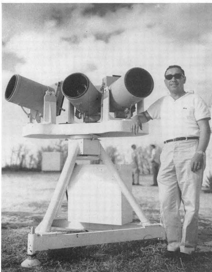
BALLISTIC PLATE CAMERAS, designed by J. S. Llamas (7224-1) recorded the RFD-1 reentry as broken streaks on 8x10-in. glass film plates. Mr. Llamas engineered the conversion of the three surplus aerial mapping cameras and associated newly-designed features for the RFD-1 flight.
