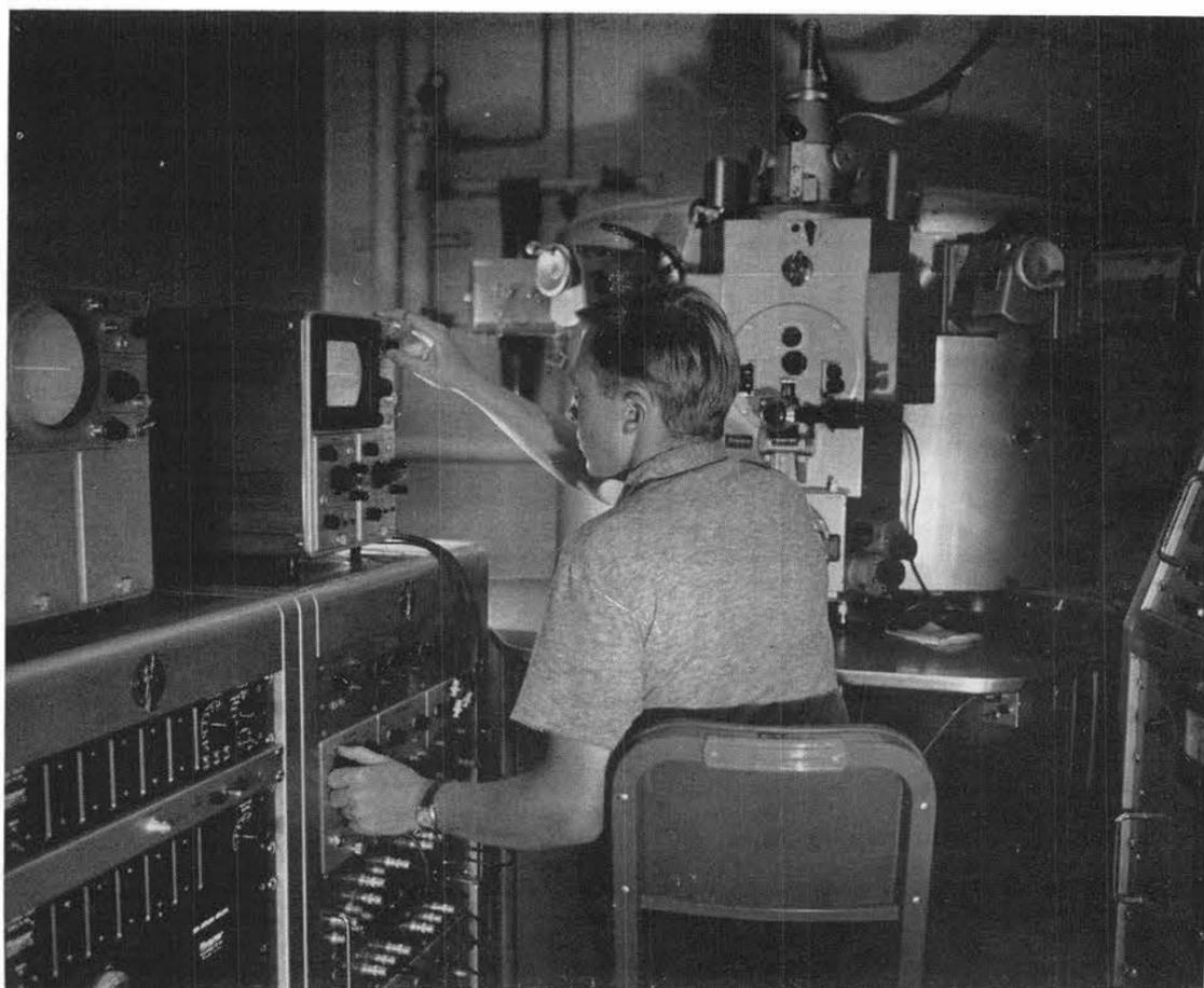
ELECTRON PROBE MICRO-ANALYZER, operated by Dave Boknecht, provides a valuable research and development tool for Sandia Laboratory. The instrument is used by Chemistry and Spectroscopy Division 1122.
