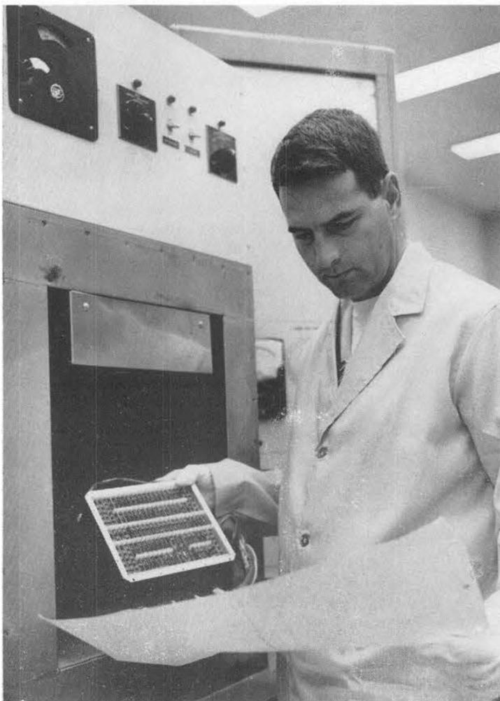
CHAMBER TEST — Ross R. French (7432-2) prepares a satellite logics system module for a temperature test. Small chamber provides heat-cold environment from -25° to +175° F. Module will also be connected with AGE tested for performance check while in the chamber.
