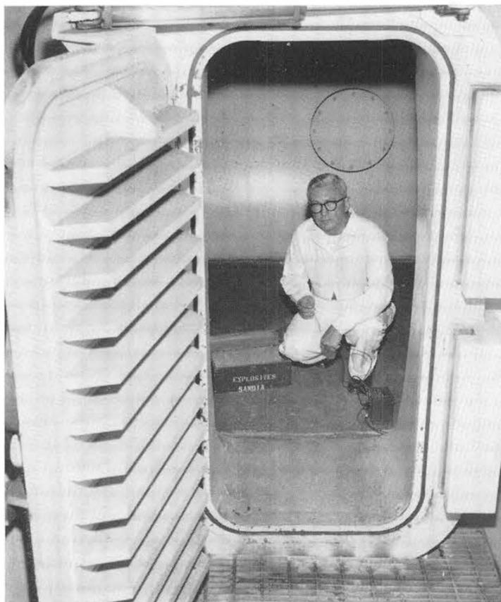
HIGH EXPLOSIVES TECHNICIAN T. K. O'Kelley (8242-1) removes mis-fired detonator from a charge inside one of the Livermore Laboratory firing chambers. The detonator will eventually be destroyed in the explosives incinerator along with other faulty explosive devices.
