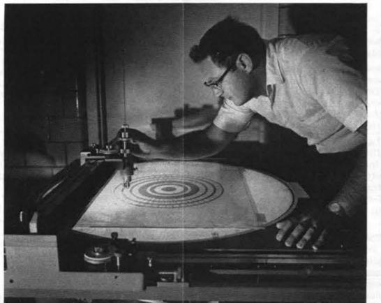
KARL D. SVENSSON (4411-5) uses this Swiss-made plotter to create a printed circuit master. The machine's extreme accuracy and rotating table are important tools in his cutting and stripping work on masters.
