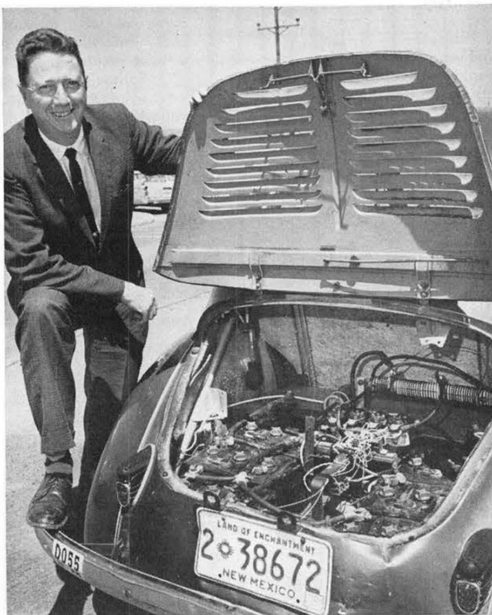
PAUL STICKLER (2543) displays the "Little Joule," electric powerplant he designed and built for his '55 Renault 4CV. The car achieves 40 mph, has a range of 17 miles, and can be recharged overnight at home.
