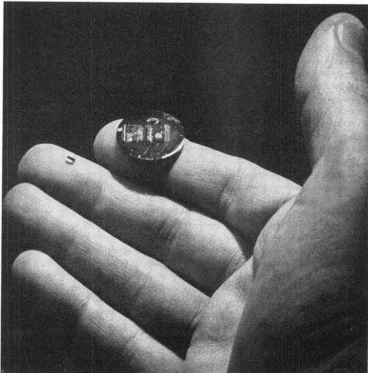
SANDIA SAMPLES — Displayed here are experimental thin film devices produced by Advanced Development Section 1433-2. Tiny speck at left contains three alloy diodes. Wafer contains field effect transistors.
