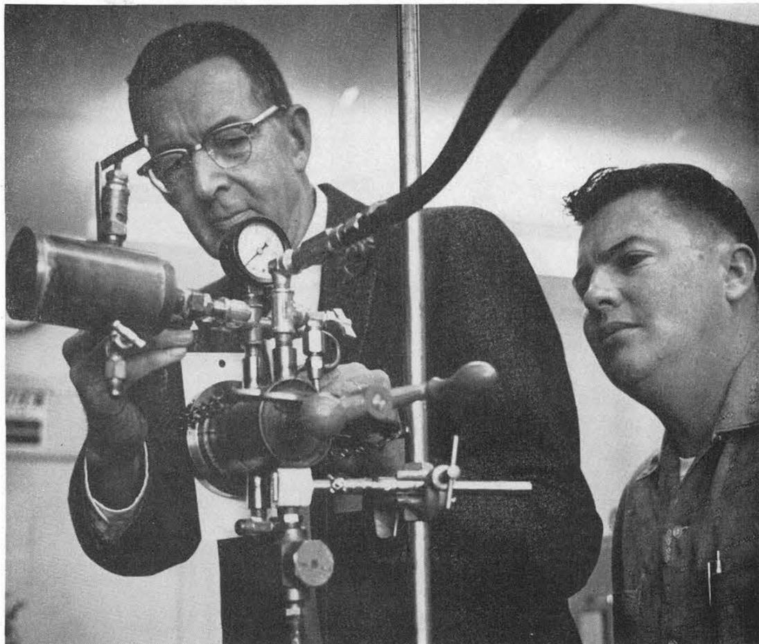
CO-INVENTORS of humidity testing device, Vernon E. Arnold and Shary D. Holmes (both 1121-1), examine prototype model of their invention. Punched metal plate beneath pressure gauge is paint sample.
