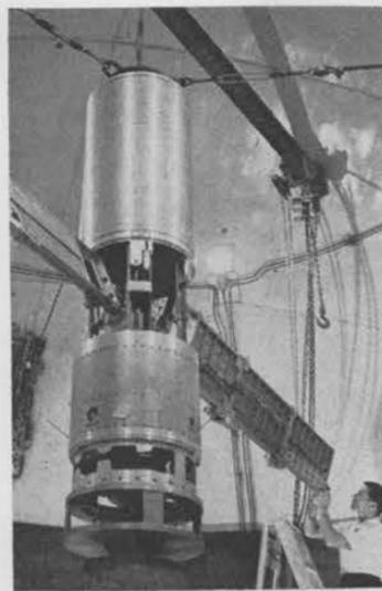
Nuclear Debris Sampler Unit Undergoes Tests
