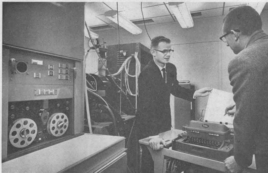
APAR - 3G machine is being used by Floyd McIver (5311), right, in a system to test performance of semiconductors prior to irradiation. At left is Bob Moyer,
