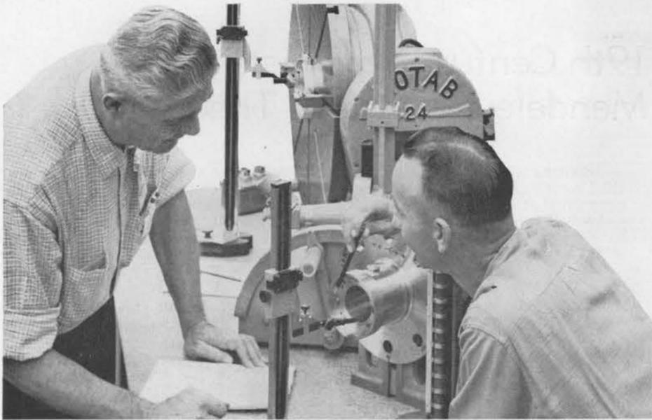
**SAFETY ENGINEERING AND ENVIRONMENTAL HEALTH DIVISION 8242:** Ray Campbell (8242-2), right, conducts test with air sampling device to determine amount of dust in air surrounding C. J. Tillman (8223-1) while machining material on lathe. Industrial hygiene, health physics, industrial accident prevention, fire prevention activities, and control of explosives, toxic, flammable, radioactive and special materials are also part of this division's job.
