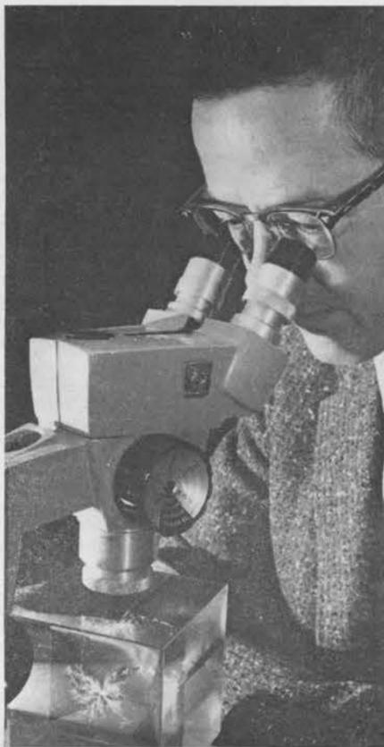
INSPECTING breakdown pattern in sample of dielectric resin used for "potting" electronic components, Osborne Milton, supervisor of Dielectric Materials Properties Section 1112-2, uses binocular microscope. The "tree" pattern visible in the center of the sample block grows from the tip of an electrode embedded in resin as high-voltage electrical current is pulsed through it.
