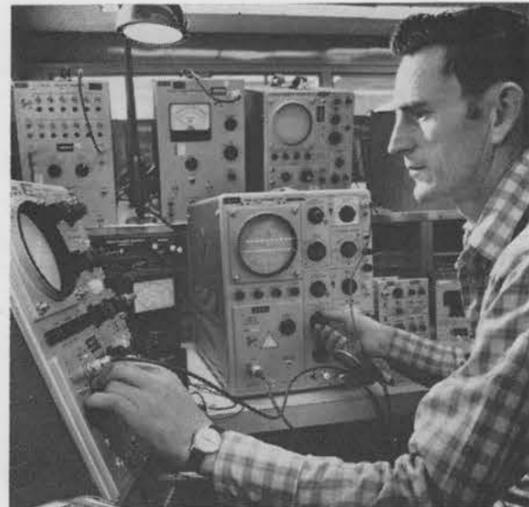
USING ONE OSCILLOSCOPE as a comparator, Alvin Plant (4233-3) calibrates another oscilloscope in electrical standards laboratory. Complete training in secondary standards calibration techniques is part of Electronics Apprenticeship Program. A Sandia employee for six years, Alvin came to the program from Janitor Services Division.
