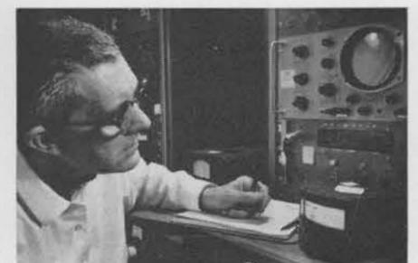
A TRANSFER STANDARD is being used by Harold Badersted (4632-2) to calibrate a voltmeter.
