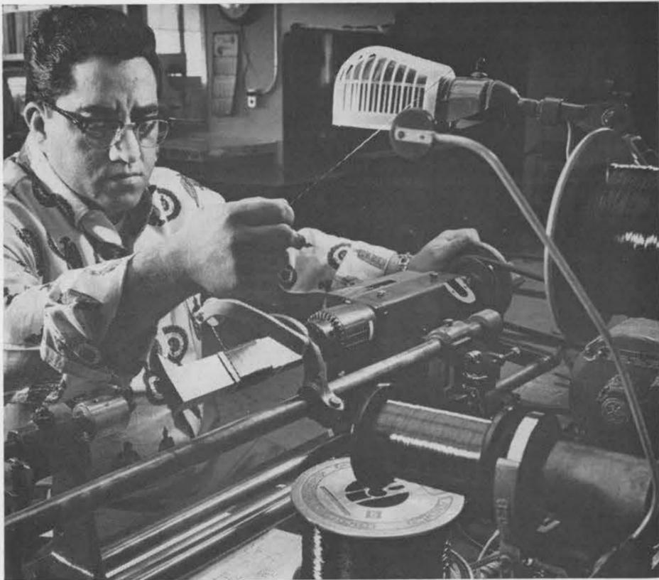
WINDING a transformer core, Fidelino Carrillo (4233-2) carefully hand-turns copper wire on winding machine in Transformer Shop. In addition to transformer and capacitor theory, he learned to prepare coils of any conceivable type, from tiny, donut-shaped helical coils to kilowatt-sized transformers. He began his Sandia career seven years ago, and came to the Electronics Apprenticeship program from Assembly Section 4233-1. He's one of six graduates.
