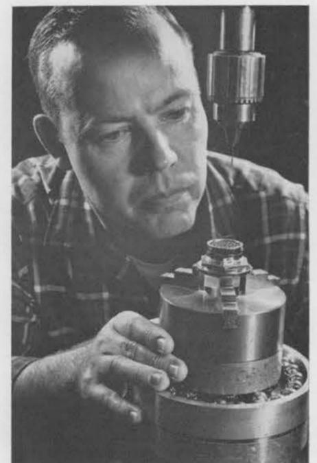
REPEATED TESTING to determine the contact and engaging forces in connectors is the purpose of this machine, operated by Gerry Hinman (4632-2). The mechanical design of connectors is important to the reliability of nuclear weapons. The force necessary to engage and the energy required to disengage individual conductors is measured through electrical transducers, and is recorded on strip charts.
