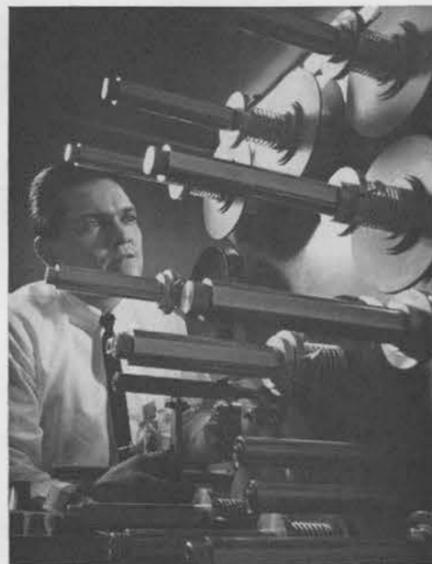
MYLAR STRIP AND METAL FOILS are wound together on this machine to fabricate an electrical capacitor. Lee Amador (4233-2) learned to operate such equipment with a variety of materials, as well as to prepare miniature coils, capacitors, and other components with specialized manipulating devices. Time spent in learning shop techniques was offset by hours of theory study. Lee came to the Electronics Apprenticeship program from Documents organization. He's been at Sandia Laboratory for five years.
