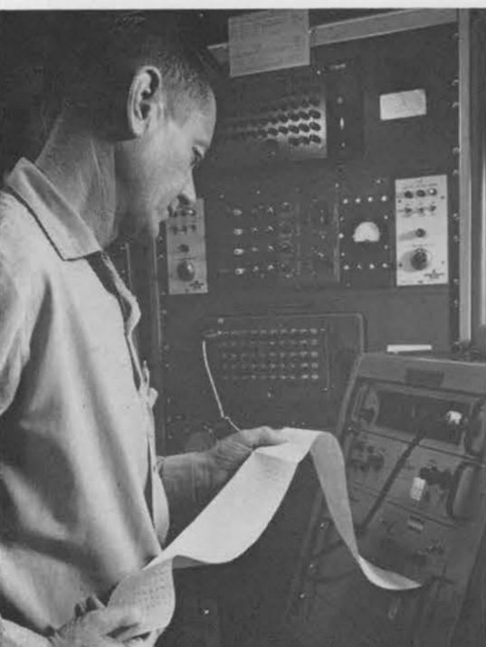
A "PRINT OUT" on the progress of indefinite run tests on resistors under power loads is being studied by Ormand Williams (4632-2). Electrical loads can be applied, along with temperatures up to 195° F.
