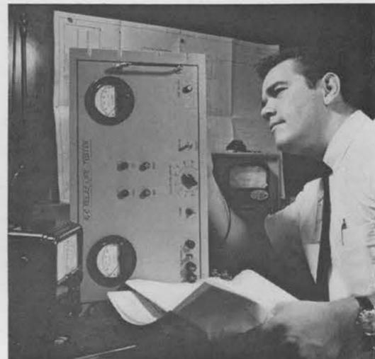
CHECKING OUT a relay life tester built by electronics apprentices, James Lujan (4233-2) uses a volt-ohmmeter. In addition to their study of the theory and assembly of electronic equipment, apprentices learn to operate a variety of electronics test equipment, and to interpret test results. A Sandian for six years, Jim came to the program from Sandia Laboratory's Printing Section.
