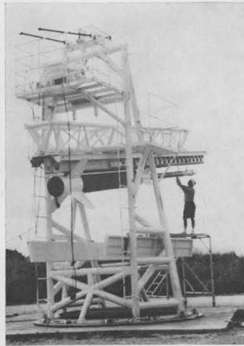
E. R. PARSONS (7214) readies a Nike-Apache rocket at Barking Sands launch site. Launcher is at work position and will be raised to vertical position for firing.
