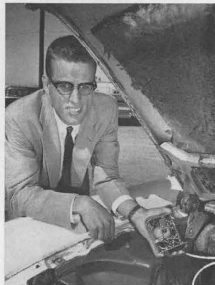
FRIEND R. BECHTEL (7252) displays his unique capacitor discharge electronic ignition system. The unit delivers a white hot spark for cold weather starts and cuts wear on plugs and points while economizing fuel.
