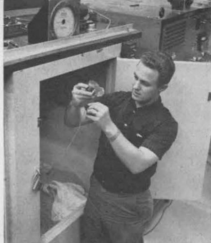
JOHN STULL (8123-3) is spending his second year in the co-op program at Livermore Laboratory where he has been assigned to work in environmental testing. Here he prepares to place a projectile in the Laboratory's electro-magnetic shock facility. He has also designed and developed an automatic timer and operating control.
