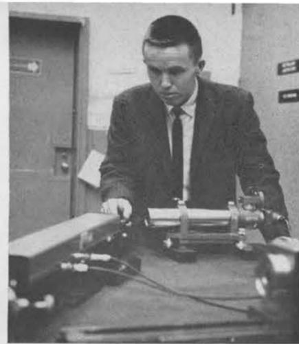
LASERS occupy the interest of Jeff Edixon (8151-1), who is completing his last period in the co-op work-study program at Livermore Laboratory. The laser is being developed for use as an interferometer, a sensitive measuring instrument.
