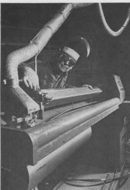
POSITIONING a cylinder on the automatic longitudinal welding machine, Leslie Cox completes setup operations. The machine automatically completes welding process.
