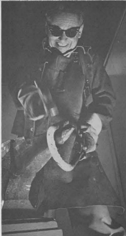
MOST MODERN of welding shops, such as Sandia's, must occasionally use ancient techniques of metalworking for a particular job. Fred Buttrey hand-shapes a part using hammer and anvil. Piece was torch heated.
