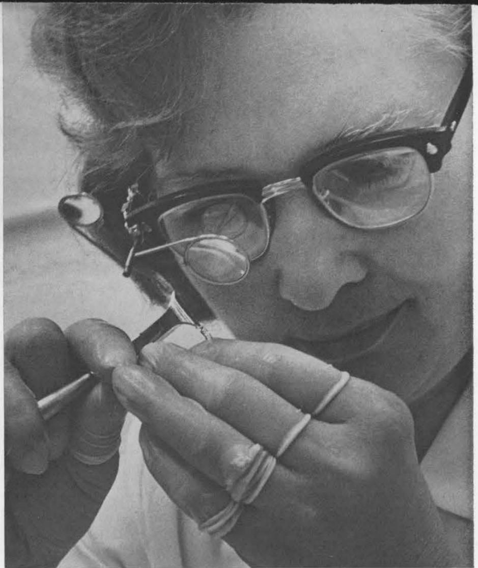
PRECIOUS MATERIALS are put to a variety of scientific uses at Sandia Laboratory. Some of the materials, in the form of precious metal alloys, are used for brazing purposes. Mayme Brunacini (4233) prepares tiny coil of gold-silver-copper brazing alloy.
