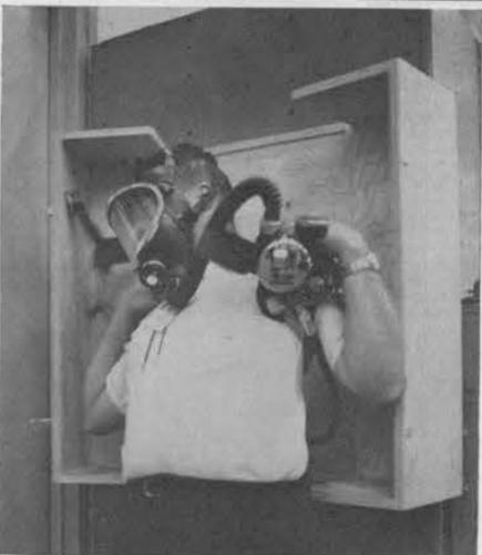
A. E. HALL shows how the air-pac container, mask, and valve are mounted in the opened wall-hung box, then demonstrates how rapidly he can get into the safety gear.
