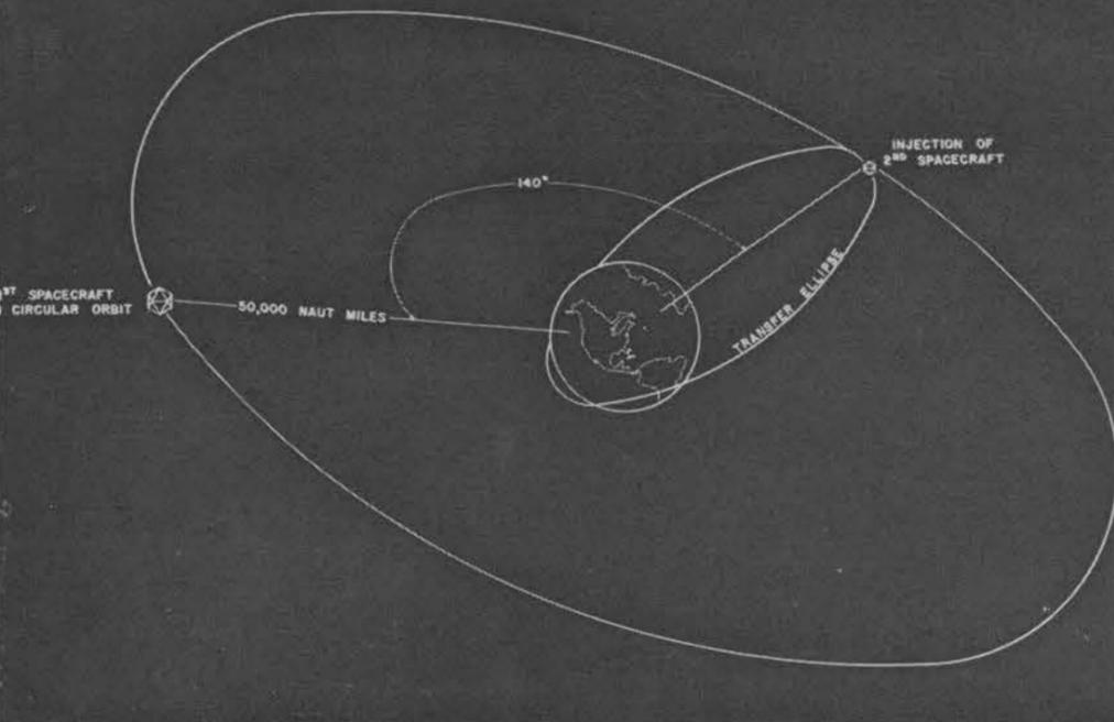
DETECTION SATELLITES' orbits are shown in this drawing. From the transfer ellipse, both satellites were accelerated into the circular orbit, but the second followed the first after traveling the transfer ellipse twice, some 40 hours later.
