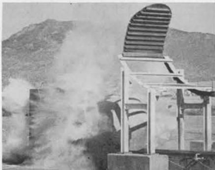
TANK EMPTIES and water fills target block containing test items.
