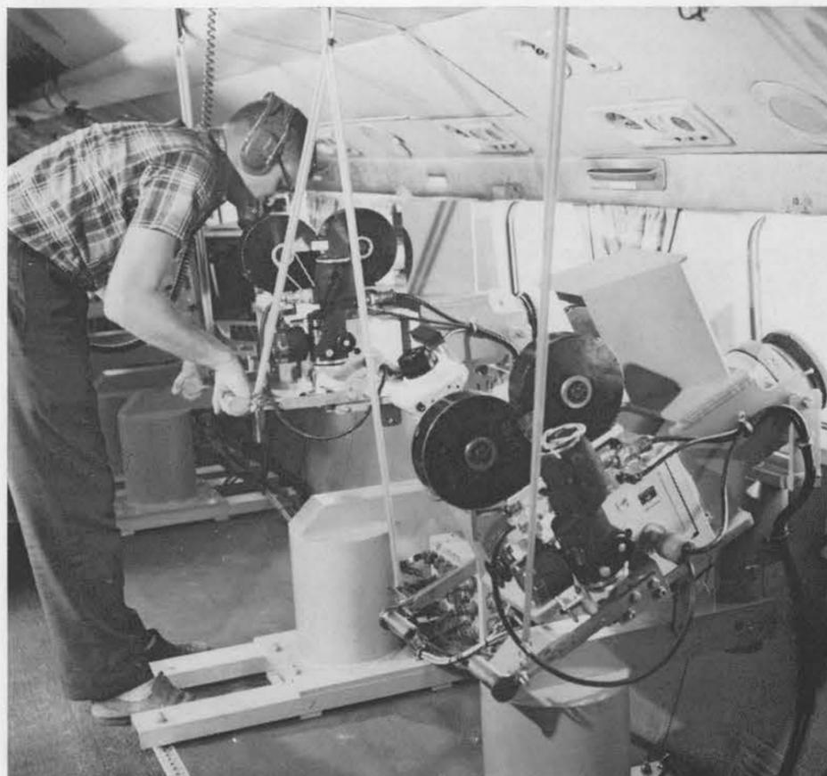
BILLY MARSHALL checks one of the high speed motion picture cameras inside the DC-7. Most of the 25 cameras on board will operate automatically with a fixed field of view. Others will be manually operated to track reentry and burnup of the RFD-2.
