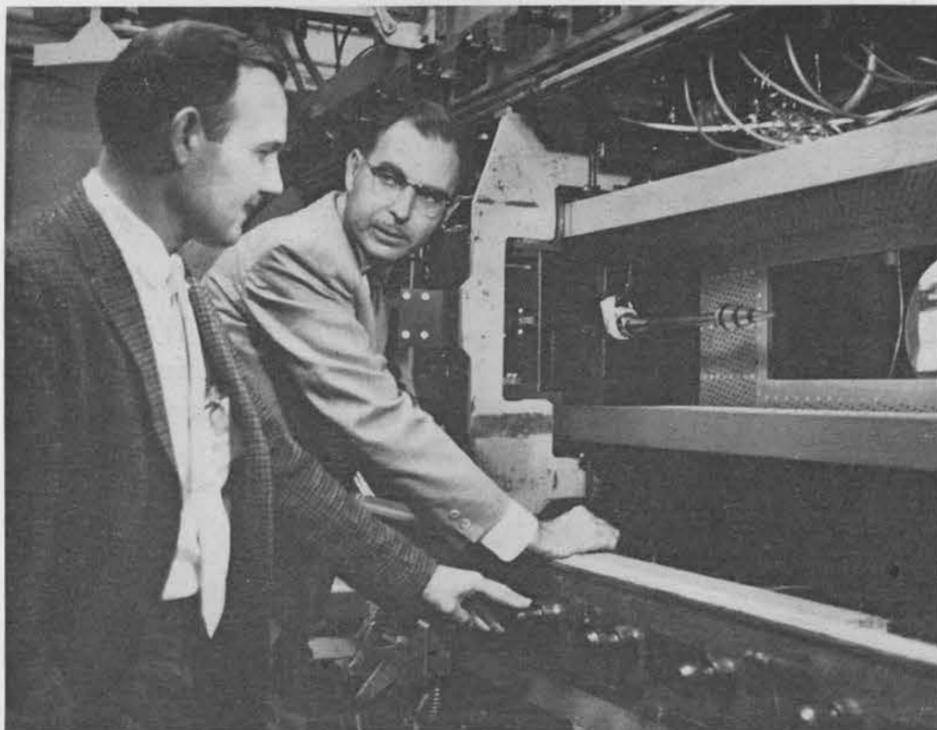
AUTHORS Kenneth L. Goin (left) and Alan Y. Pope are checking over an experimental shape in Sandia Laboratory's supersonic wind tunnel.
