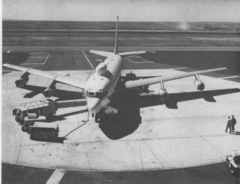
**DIAGNOSTIC AIRCRAFT**—A C-135 jet transport assigned to Sandia Corporation will carry data-gathering instrumentation during forthcoming test readiness exercise in the Pacific. The aircraft is one of three "flying diagnostic laboratories" outfitted with instrumentation normally mounted in ground installations. One of the purposes of the exercise is to test airborne diagnostic techniques.
