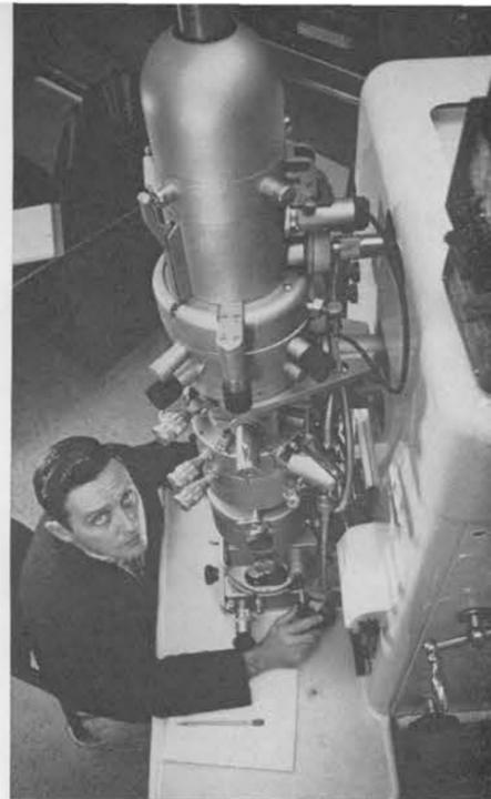
ELECTRON MICROSCOPE, operated here by A. W. Mullendore of Sandia's Analytical Methods Section II, is used to explore and inspect the smallest details of the surfaces and inner structures of a variety of materials. The upper part of the instrument is an electron "gun" used to produce and direct a beam of electrons to the specimen under study and through magnetic "lenses" to an observation point.
