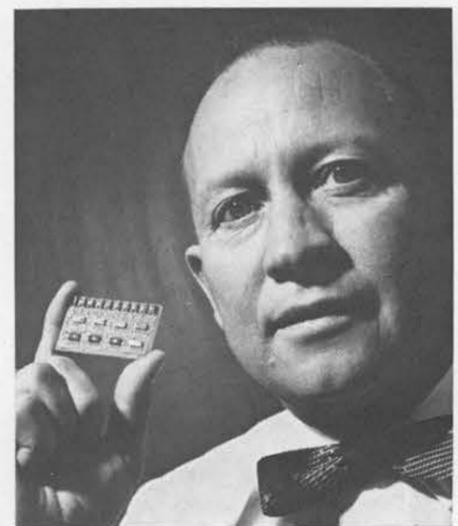
INTEGRATED CIRCUIT MODULE for the Vela Hotel detection satellite is displayed by N. A. Cordova, supervisor of Sandia's Printed Circuitry Section. Raised rectangles on the printed circuit board are components of different functions which can be combined in many ways to form a desired system.
