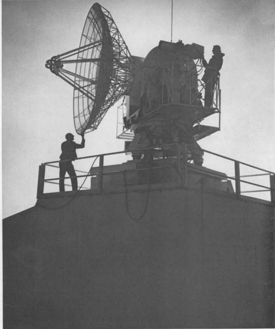
SILHOUETTED AGAINST AFTERNOON SUN is an AN-MPS-25 radar, located on Radar Hill some 700 ft. above the dry lake which comprises the main target. The one megawatt radar has a maximum range of 500 miles and a 12-ft. diameter parabolic reflector. Operators are Grant Gardner, left, and Bill Moore, Special Facilities Section.
