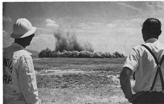
COYOTE TEST FIELD at Sandia Laboratory's back door has served as an outdoor laboratory in the study of excavation by explosives. Small charges of conventional explosives tell scientists what might happen if nuclear devices are used to move earth.
