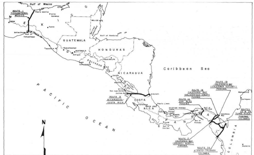
TRANSISTHMIAN ROUTES—Studies reveal several possible routes for nuclear-excavated canals. It has been determined that if canals would be dug by such means, excavation costs could be reduced as much as 90 per cent and the total cost by as much as 65 per cent.
