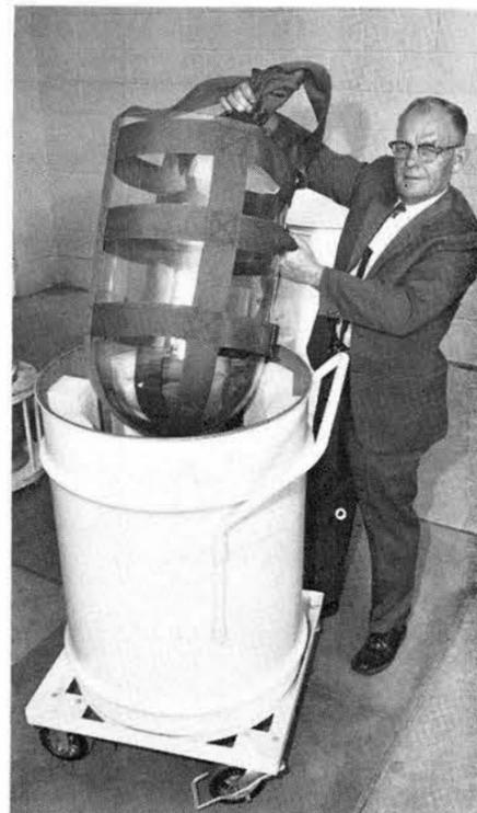
E. R. WOOD of Physical Electronics Section displays his new safety system for moving and handling large, glass, laboratory bell jars. Converted A/N can has wheels, handle, and foam cradle inside.
